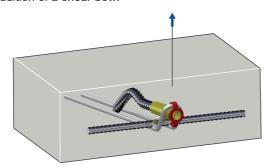
Shear load can be increased by using shear bow reinforcement.
