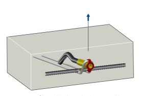
Shear load can be increased by using shear bow reinforcement.
